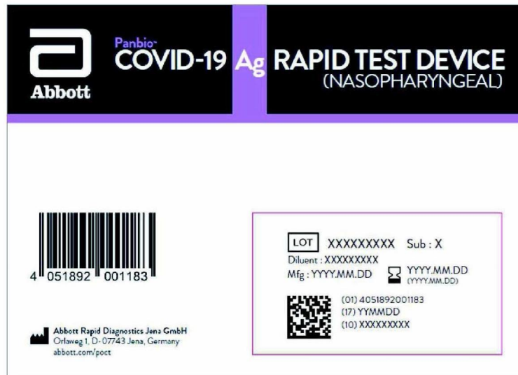
Figure 2-10: Panbio™ COVID-19 Ag Rapid Test Device Ref. 41FK10 specific label information: Manufacturer name and address and label information (incl. storage conditions, lot number, expiry and manufacturing dates, UDI information)
